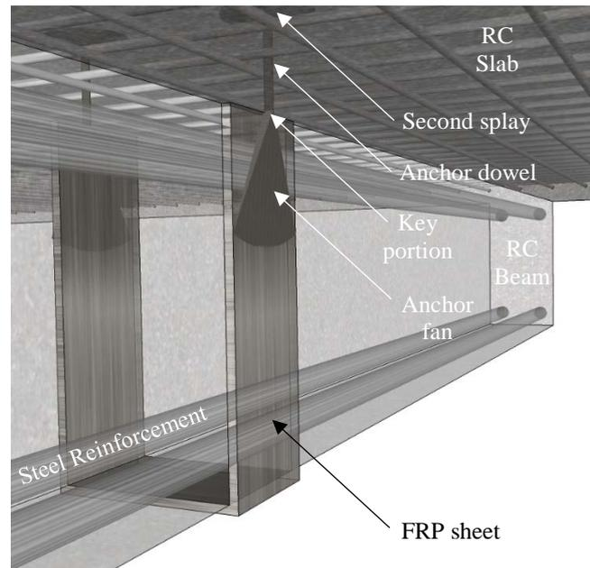
Figure 1: Graphic representation of an FRP U-wrap anchored with a straight FRP anchor
