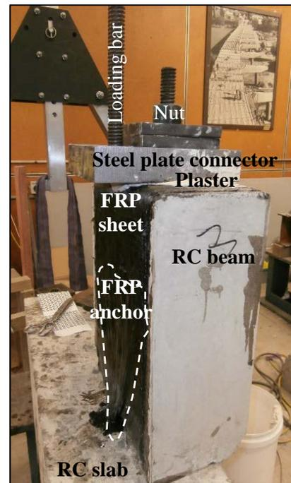
Figure 2: Test set-up
