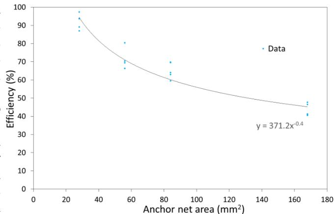
Figure 3: Strength efficiency of anchors with varying net-fibre area
